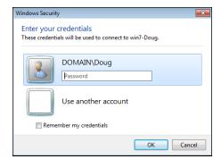
FIGURE 2-3: Logging in to a remote computer.
